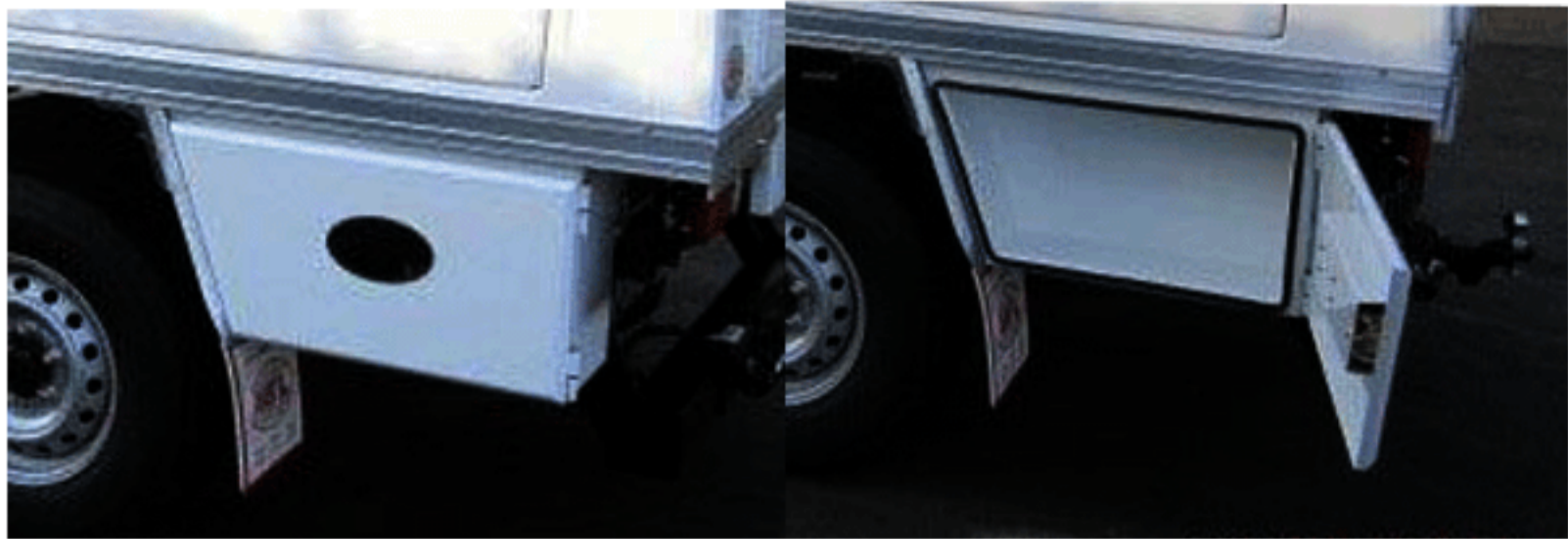
Steel Powdercoated white or black LF/RR RF/LR options Dimensions: 29.5L(top) 23.75 (bottom) x 16H x 9.75 deep or 25.5 (top) 19.8 (bottom) x same H/Depth
